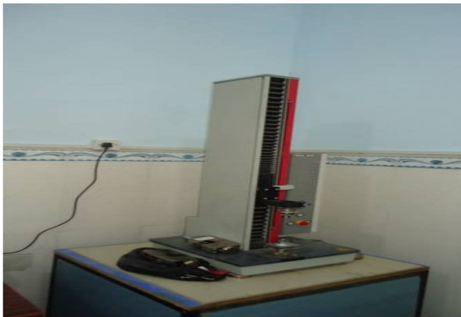
Figure 2: Tensile test of the specimens was carried out with a Zwick/Roel type [BT1-FR2.5 TN.D14]
